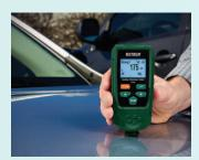
Dual technology provides automatic recognition for ferrous and non-ferrous substrates without having you guess the material. Allows for quick, one-handed operation for non-destructive measurement of the coating thickness on various surfaces.
